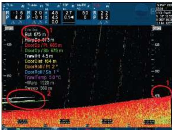
(1) Without correction for temperature: depth shows 675 m.
